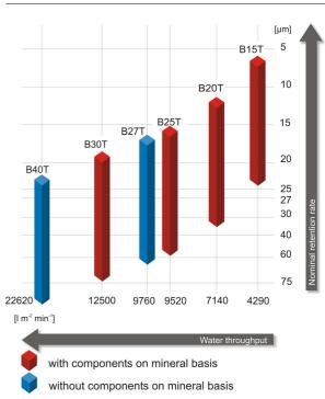
Conditions: $\triangle$  p - 100 kPa (14.5 psi), medium: water at 20 °C (68 °F)
