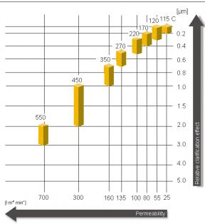
Conditions:  $\triangle p$  -100 kPa (1 bar), medium: water at 20 °C (68 °F)
